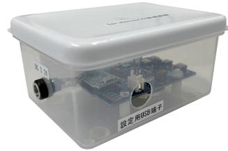
図4 Sensor-based Regulation Profiler Synchronizer
